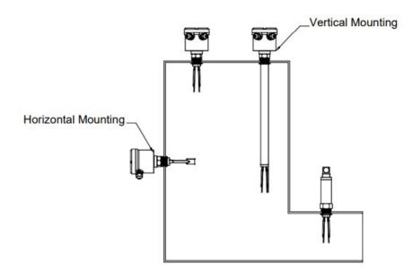
Figure 3 : Mounting Arrangement
