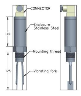
Figure 2 : Vibrating fork ( Pipe Fork )
