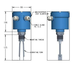
Figure 1 : Vibrating fork level switch
